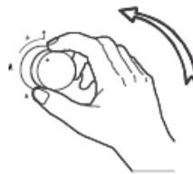
While holding down the button, lighter steps in and starts to ignition.
