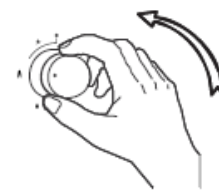
By turning the button left while holding down, you can provide ignition at flame length you want.
